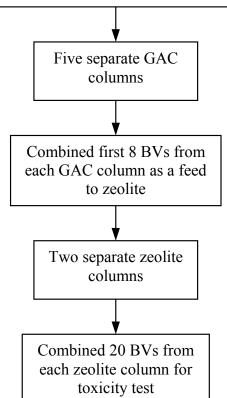
Figure 4 Flowsheet of Bench-scale GAC + Zeolite Treatment Evaluation
