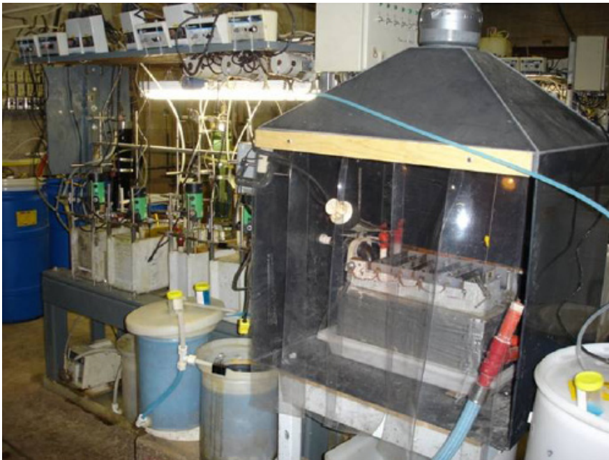
Figure 7: The Copper Solvent Extraction and Electrowinning Section
