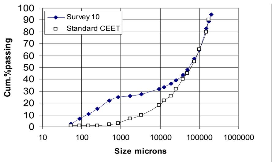
Figure 1: Typical AG feed size distribution as measured compared with Rosin-Rammler distribution generated within CEET
