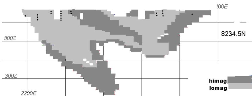
Figure 3: Section through Luce showing ore types
