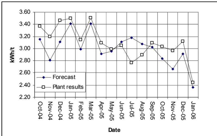
Figure 7: Comparison of plant energy usage with that expected from actual ore blocks mined Oct 04 to Jan 06
