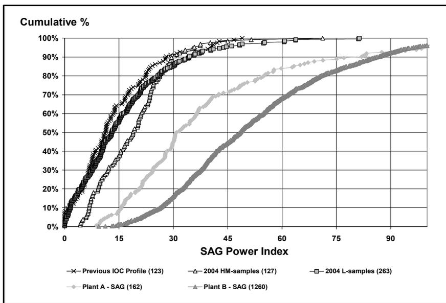
Figure 2: Comparison of the distribution of SPI values for IOC ore bodies with other soft to medium ore
