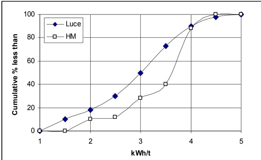
Figure 6: Distribution of energy requirements for blocks in each ore body
