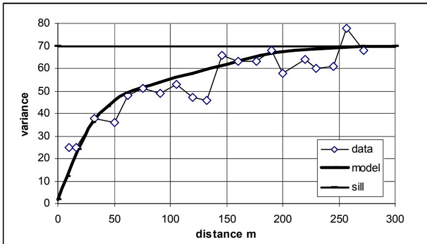
Figure 4: Variogram for SPI values in Luce ore body
