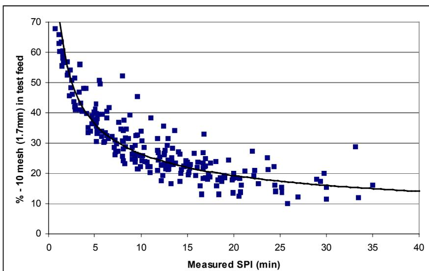
Figure 9: % minus 10% in SPI test feed vs. SPI value
