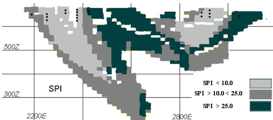
Figure 5: Section through Luce showing estimated SPI values for blocks
