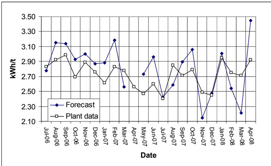
Figure 8: Comparison of plant energy usage with that expected from actual ore blocks mined July 06 to April 08
